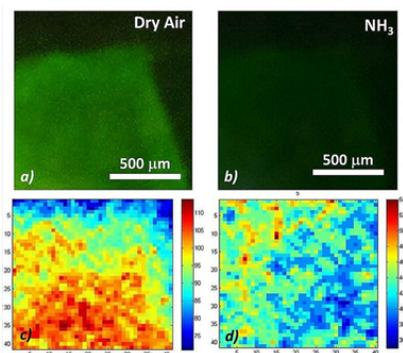
**Figure 3.** fluorescent fibers UV-LED irradiated before (a) and after exposure to a few ppm of NH<sub>3</sub> for 20 min (b); image analysis of the GREEN matrix of pixels (among RGB matrices) before (c) and after gas exposure (d)
