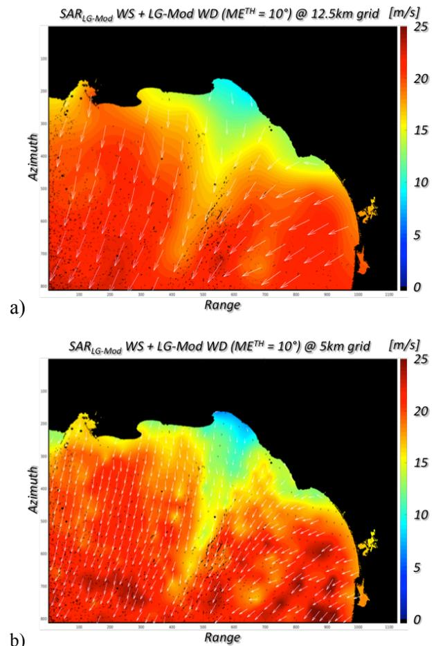
**Figure 1. SAR LG-Mod wind directions (white arrows) and corresponding CMOD5.N wind speeds (coloured background) from a Sentinel-1 IW image, 5<sup>th</sup> Feb 2015, at (a) 12.5 km and (b) 5 km grid. Reliability threshold for directions selection  $ME^{TH}=10^\circ$  (and  $\alpha=0.05$ ). Unusable pixels masked in black**
