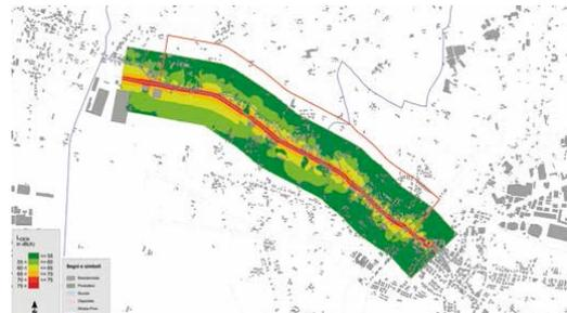
**Figure 1. Example of an acoustic map**
