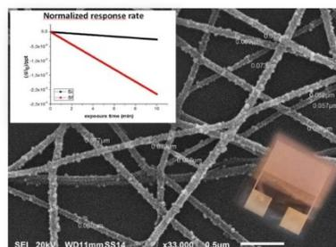
**Figure 1. Fiber AuNPs decorated (SEM). Inset: a fibrous coating on IDEe current changes when Hg<sup>0</sup> was injected and flowed over the sensor**
