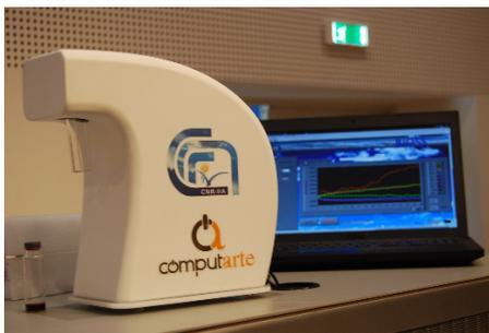
Figure 5. Prototype of an Electronic Nose based system for smart wine analysis (photo taken during an event held in EXPO 2015)
