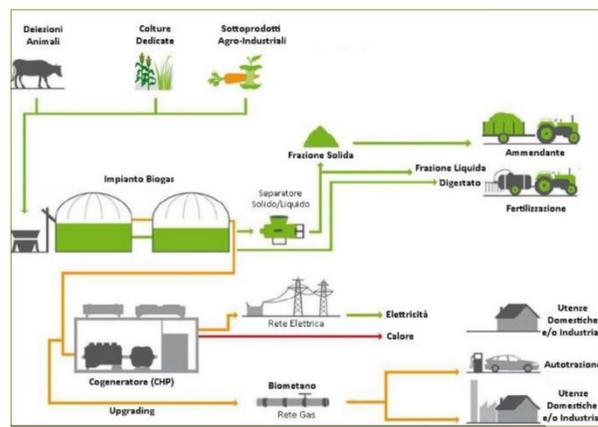
Figure 2. Typical biogas production scheme
