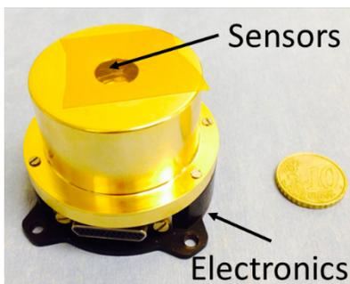
Figure 4. CAM Sensor Head.
