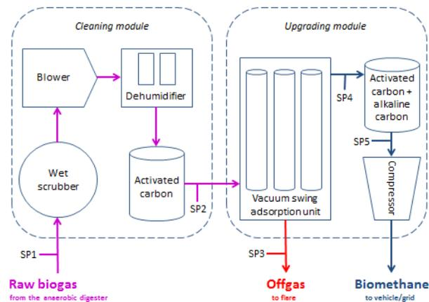
Figure 3. Biogas upgrading unit in Milan
