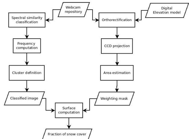
**Figure 2. Description of the image processing required for estimating the fractional snow cover area**
