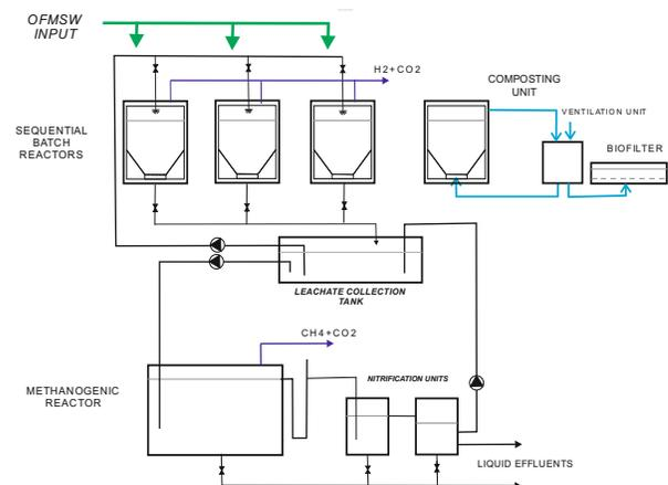
Figure 1. Schematic of the anaerobic digester
