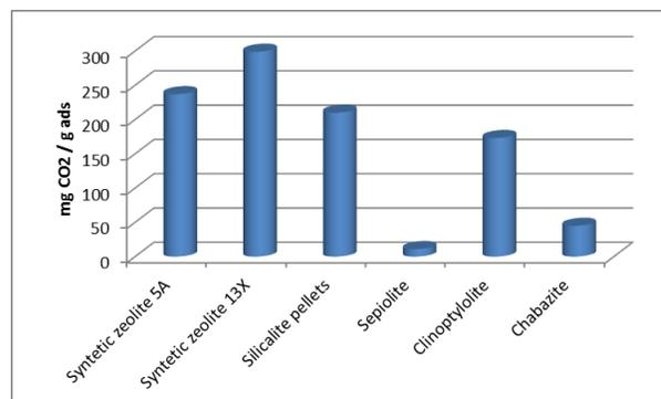
Figure 4. Adsorption capacity of zeolitic materials
