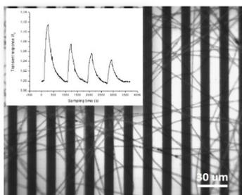
**Figure 2.** Optical micrograph of IDE electrodes coated by PHB-PS-Graphene fibers. Inset a plot showing transient responses to decreasing concentration of NO<sub>2</sub>
