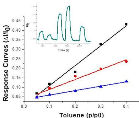
**Figure 1.** Response curves of PS/PHB/MGC sensor to increasing concentration of toluene when temperature increased (black square: 40°C; red sphere: 60°C; blue triangle: 80°C). Inset: plot of transient responses to various percentages of toluene vapours
