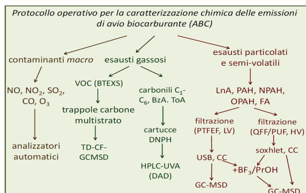
Figure 1. Scheme of analytical procedure
