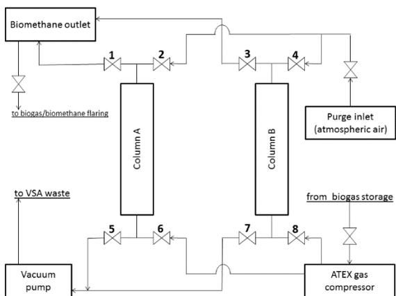
Figure 2. Schematic of the biogas upgrading unit
