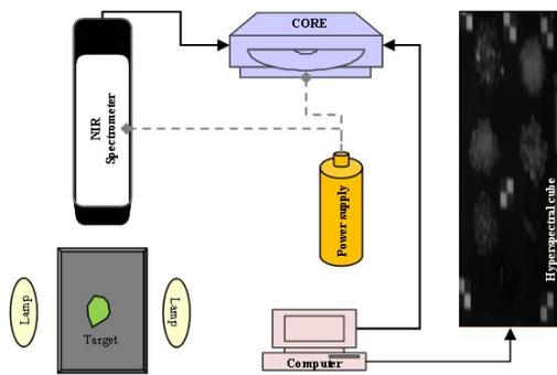
Figure 1. Diagram of the hyperspectral device
