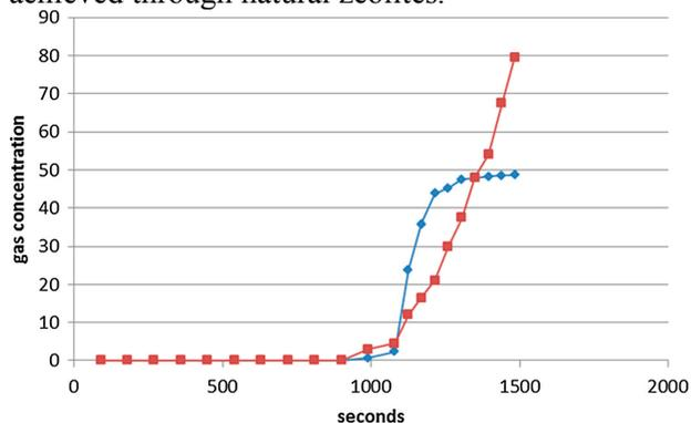
Figure 3. Outlet concentration of CO<sub>2</sub> (%v/v, red dots) and H<sub>2</sub>S (ppmv, blue dots)
