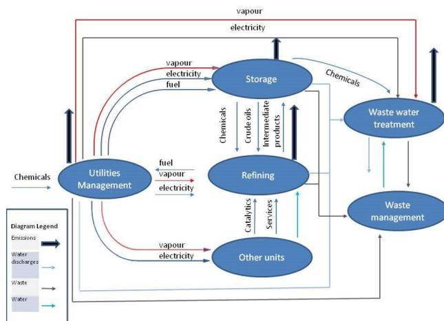
Figure 3. Raw material and energy consumption fluxes in a refinery where the thermal recovery is maximized (AIA Portal, 2015)
