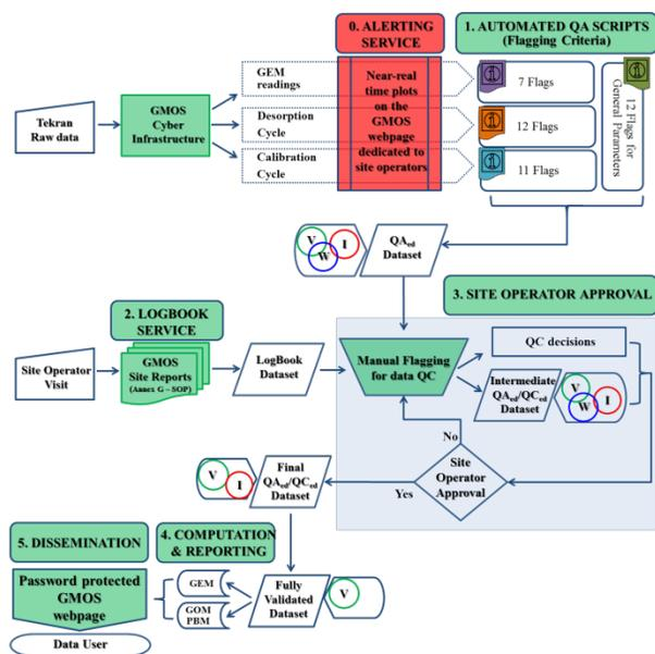
Figure 1. G-DQM workflow with the main step processes on which it is based
