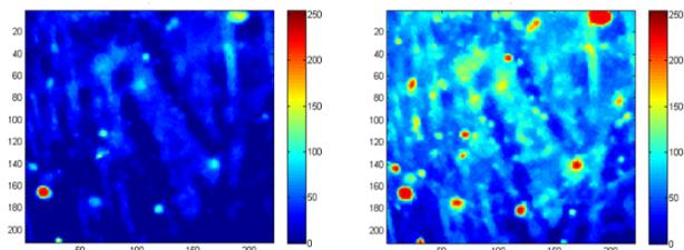
**Figure 2.** Image Analysis of green luminescent intensity of fluorescent fibers UV-LED irradiated before (left) and after (right) exposure to a 0.16 p/p<sub>0</sub> of toluene for 10 min
