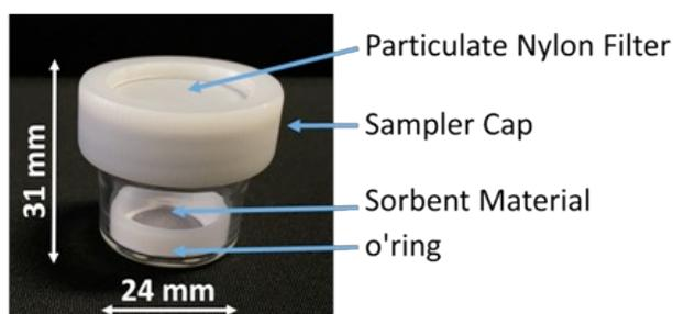
**Figure 1. Prototype of Hg Passive Sampler**
