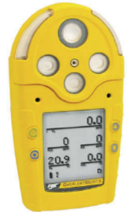
Combined Photo-Ionisation Detection (PID) and gas monitoring system.
