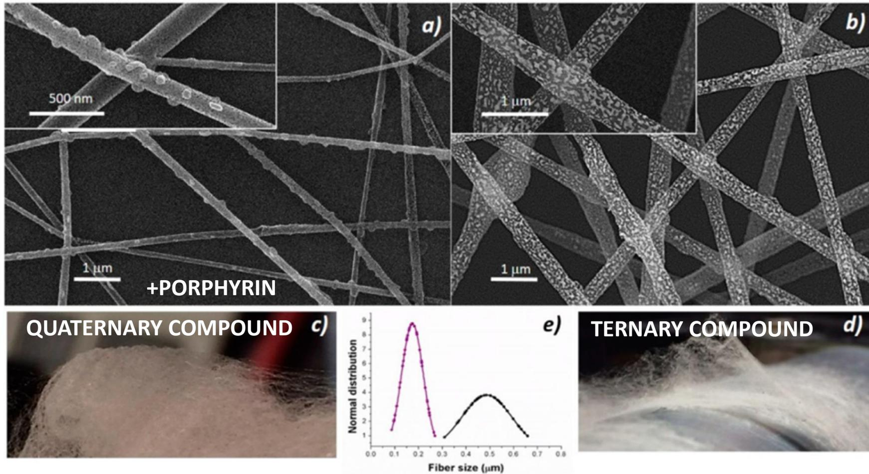
**SEM micrographs** of H<sub>2</sub>TPP-PsB-MGC (a) and PsB-MGC (b) and their respective pictures placed under (c,d). Diameter distribution graph (e) of H<sub>2</sub>TPP-PsB-MGC (purple) (a) and PsB-MGC fibers (black) (b).
