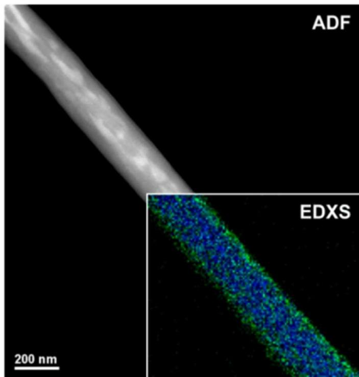
Annular dark field mode-scanning - transmission electron microscopy image of a porphyrin doped fiber. The inset shows the corresponding energy dispersive X-ray spectroscopy (EDXR) chemical map from carbon (blue) and oxygen (green).
