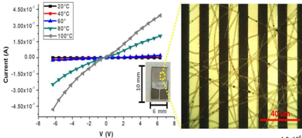
Current-Voltage curves at different temperatures (20, 40, 60, 80, 100°C) for the fibers coated IDE (inset) are plotted.
