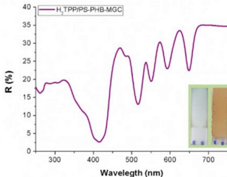
Diffuse reflectance ultraviolet-visible (DR-UV-Vis) spectrum of a  $H_2TPP$  PsB-MGC thick fibrous layer (the orange one in inset). Inset shows also a porphyrin-free fibrous coating (the white-grey one).
